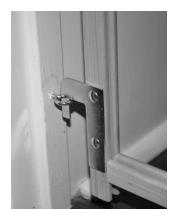
10) Swing and expand the gate and insert the bottom hooking L-bracket (Figure 10) on the gate into the bottom screw eye.
